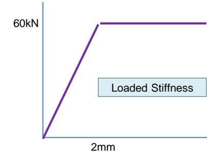
In case when Multi-linear link changes from 'unloaded' to 'loaded'.
