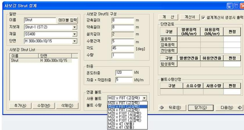
▶ 작용전단력 :  $S_{max} = P_{max} \times \sin \theta = 243.325 \times \sin 45 = 172.1 \text{ kN}$
