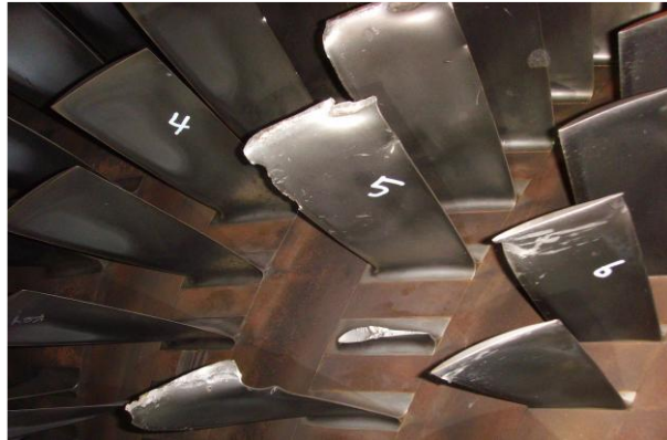
Example 1) Fatigue fracture of a blade of the compressor of the gas turbine
